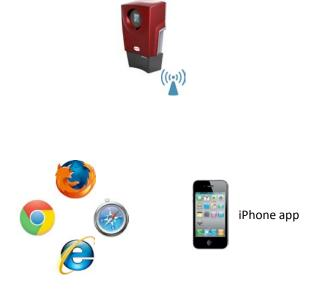
The Sunway MXS inverters are able to create an ad-hoc Wi-Fi network without using any additional devices.
