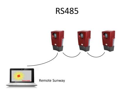
The laptop where the Remote Sunway is installed is to be connected to the inverters via RS485 through a multidrop network.
