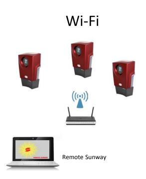
The laptop where the Remote Sunway is installed is to be connected to the same Wi-Fi network as the inverters', either an ad-hoc or a managed network.
